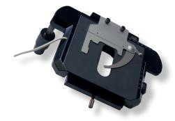
When installing a heating system in the original stage is not an option, we offer a clamp-on heated stage with a very thin plate. A transversely movable stage holder is attached through a slot in the clamp-on heated stage.
