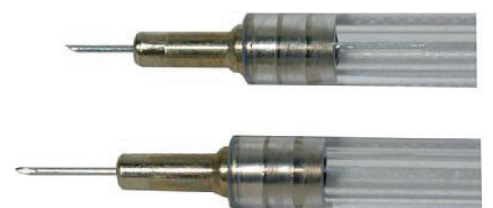
Figure 4: Different needle length of different type of Robertson pipettes (Minitube)
