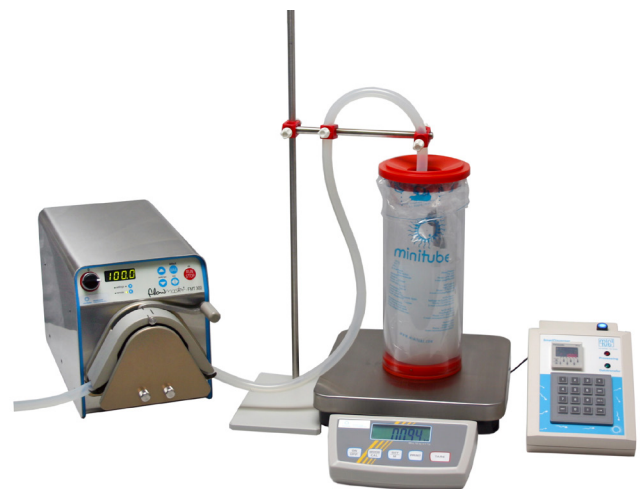
Automated semen dilution with SmartDispenser L
